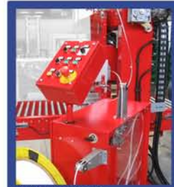
PANNELLO COMANDI OPERATOR PANEL
